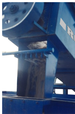
Fig. 2.- View of discharge chute of a Single Screw Washer
